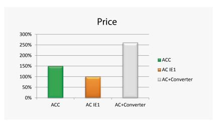
The lifecost calculation is based on 4 kW motor IE1 with 40'000 hr lifetime and 10 ct. per kWhr. The 4 kW ACC cost 200 € more as an AC motor and saves 20'0000 kWhr or 2000 € during his lifetime; the payback time is equal to 4000 hr or one year of operation. The value of the saved energy is four times higher as the ACC-sales price.
